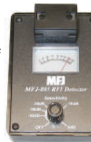
MFJ-805 Super-Sensitive RFI Sniffer works with mobile installations, ferreting out alternator hash, ignition pulses and microprocessor noise on feedlines and power leads. Isolate cables picking up RFI and know when you've suppressed the problem. Easy-to-use. Clamp current transformer over suspected cable or wire (up to ¼ in. dia.) to detect RFI causing common-mode currents. 2¼Wx4¾Hx1D inches fits in shirt pocket. Use 9 Volt battery. Usable VLF to VHF. Gain adjustable over 50 dB range. MFJ-805 $99.95 Ship Code A
